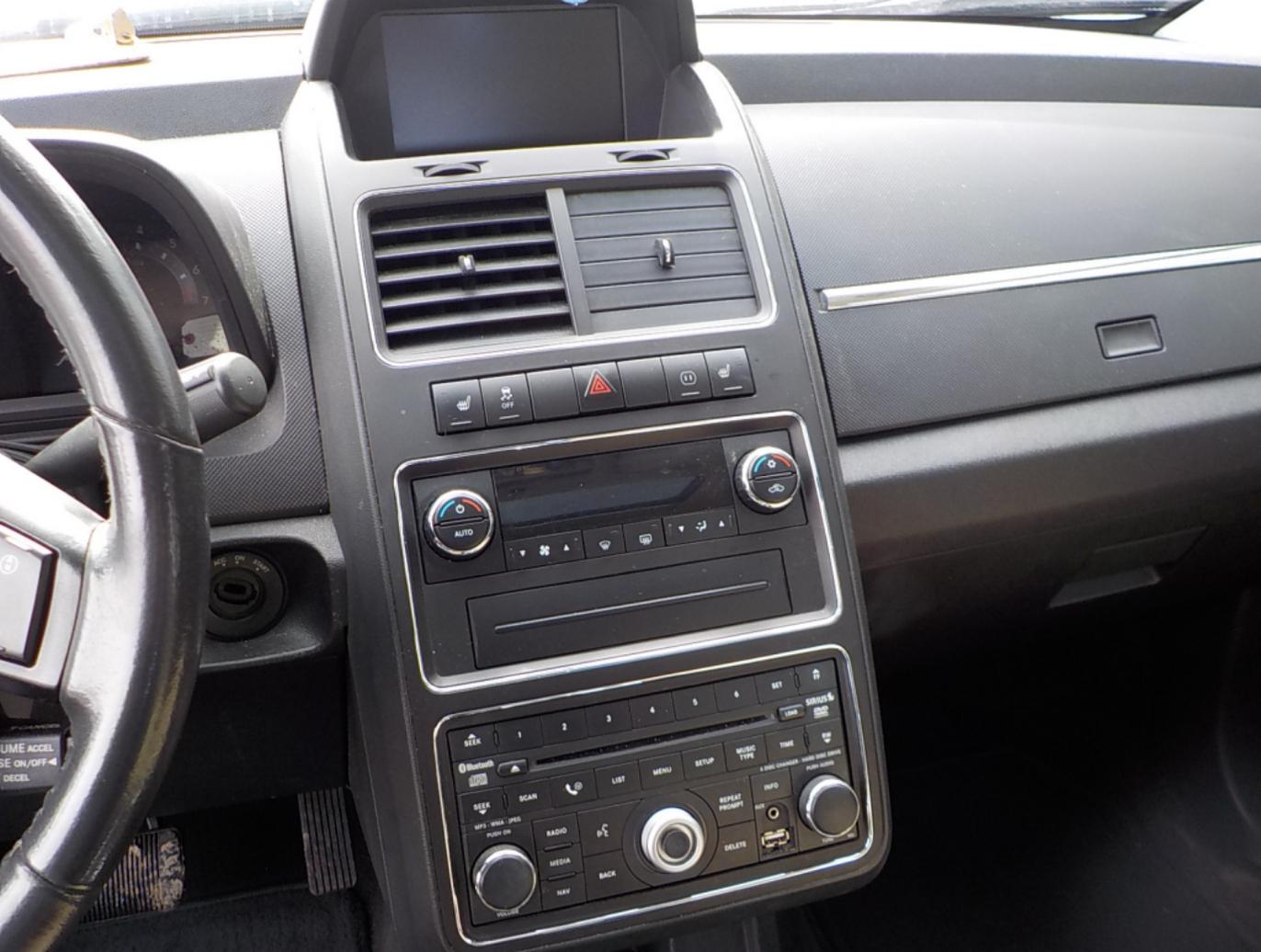
Two air vents with horizontal slats and sliding levers for adjusting airflow.
